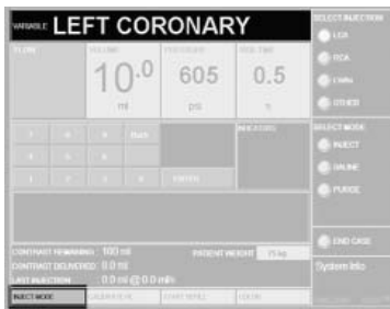
Press INJECT MODE for variable or fixed rate
