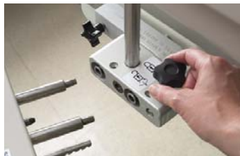
Unlock the knob by turning it counter-clockwise and pressing down
