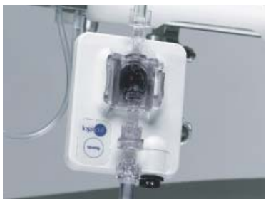
If using a transducer cartridge, connect it to the transducer backplate.
