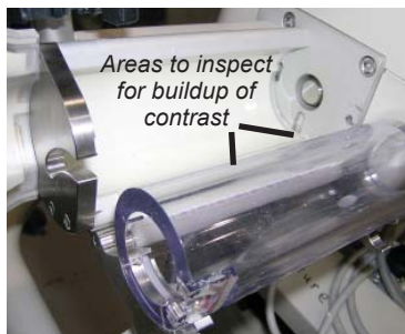
Chamber sleeve in open position
