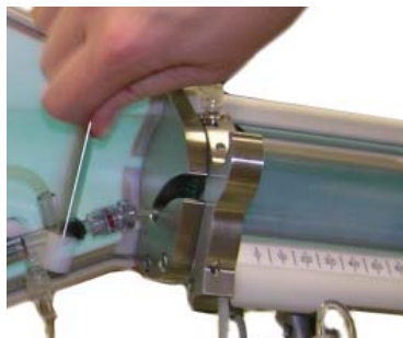
Tap the tubing with the provided mallet or a hemostat
