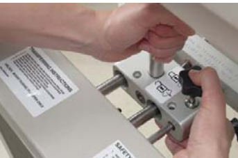
Carefully slide the injector head onto the patient table.
