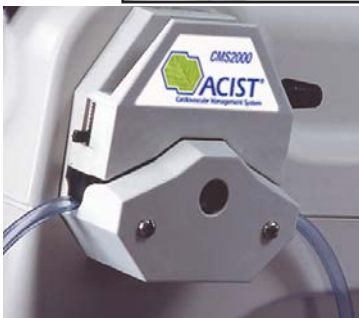
Place the saline tubing in the saline pump, making sure the black v-teeth guides are lowered on each side and centered over the tubing
