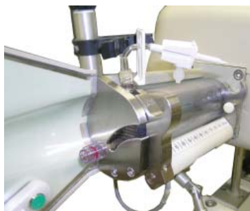
Insert the syringe in chamber and close the chamber door completely
