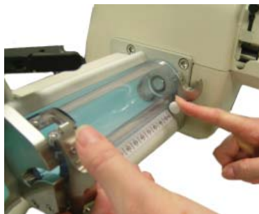
Open the chamber by pulling the white button
