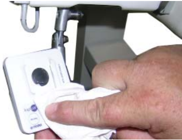
Clean the transducer backplate membrane with a damp cloth
