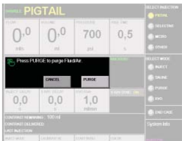
Press the PURGE button to purge air from contrast tubing
