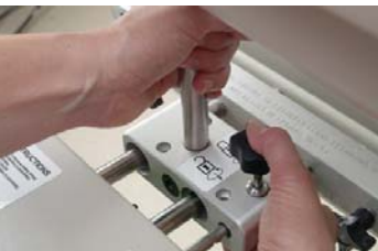
Unlock the knob on the U-Joint by turning it counter-clockwise and pressing down
