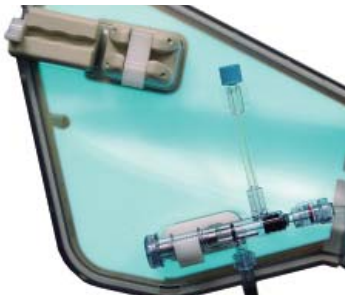
Clip manifold assembly into the manifold valve sensor
